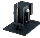
**[Scattering solids sample measurements](#)—diffuse transmittance and reflectance**
