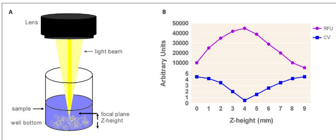
**Figure 4.** (A) Z-height is the distance between the lens and the sensing volume and determines the focal plane. (B) Performing an assay with suboptimal Z-height can result in a decrease in signal and increase in CV.
