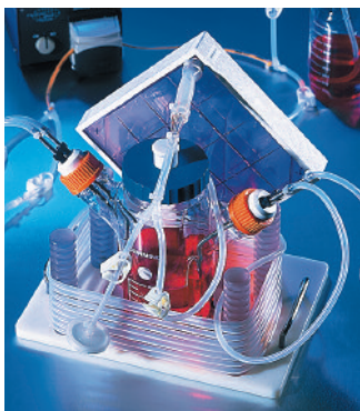
Figure 9. The Corning E-Cube system is a simple to use perfused bioreactor with an 8,500 cm 2 growth area parallel plate culture chamber.
